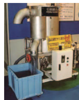
Demonstration of ozone-employed decolorization of wastewater at business show
