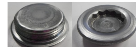
Thread-rolled parts by die forming
