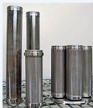
▲Hydrogen separation membrane module
