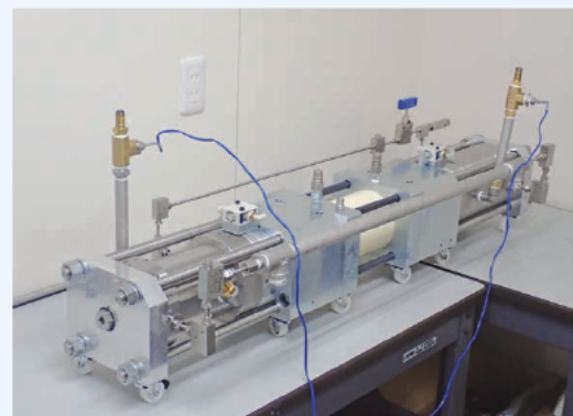
▲4Nm 3 /hr hydraulically-driven hydrogen gas booster
