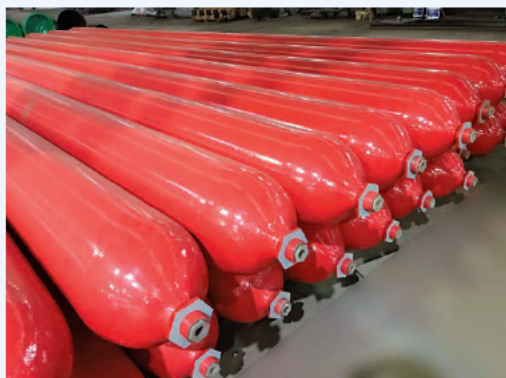
▲ Long vessels loaded on hydrogen trailers
