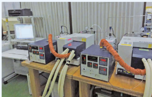
▲ Thermal analysis equipment that enables testing with various gases
