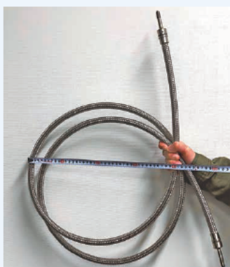
▲ Flexural state of flexible hose
