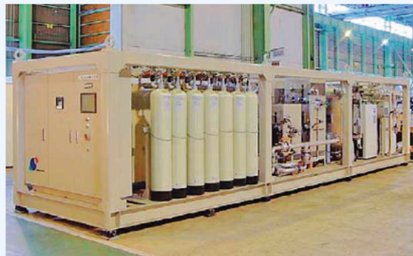
▲ Skid mounted type with improved hydrogen production efficiency
