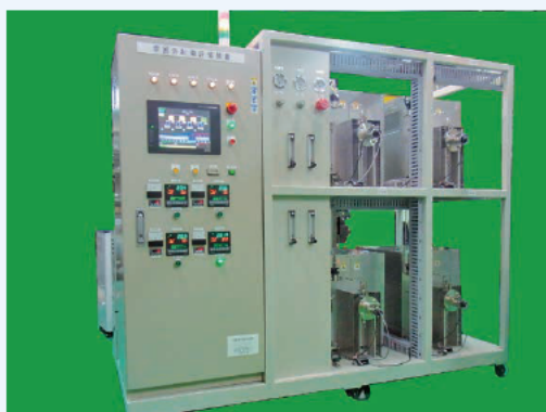
▲ Equipment to evaluate electrical characteristics in oxidation and reduction atmospheres
