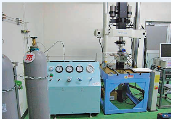
▲ Photo of the appearance of fatigue test equipment under high-pressure hydrogen
