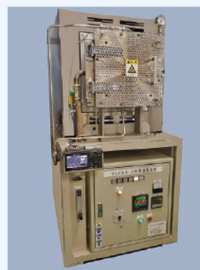
▲ High-temperature electric furnace with muffle case
