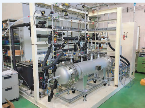
▲ Low-pressure hydrogen occluding vessel and occlusion/release performance evaluation equipment
