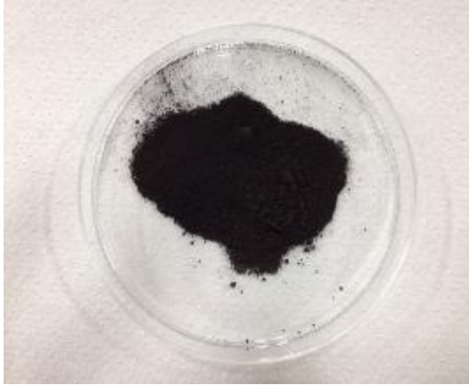
Silicon nanoparticles for hydrogen generation made from recycled industrial silicon waste
