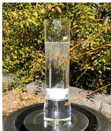
▲Water electrolyzer Height:270mm Inner diameter:50mm Electrolyte: 300cc of 10 % NaOH solution
