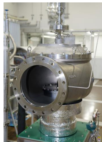
FUKUI LH2 Pressure Safety Valve
