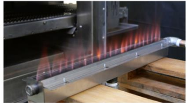
Hydrogen combustion burner developed in collaboration with Heat Energy Tech
