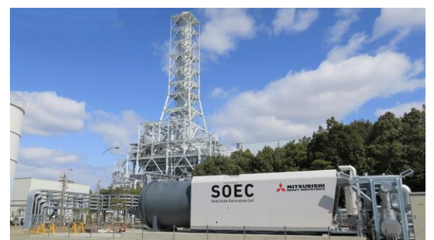
A 400kW class SOEC demonstration machine being technically validated in Takasago Hydrogen Park
