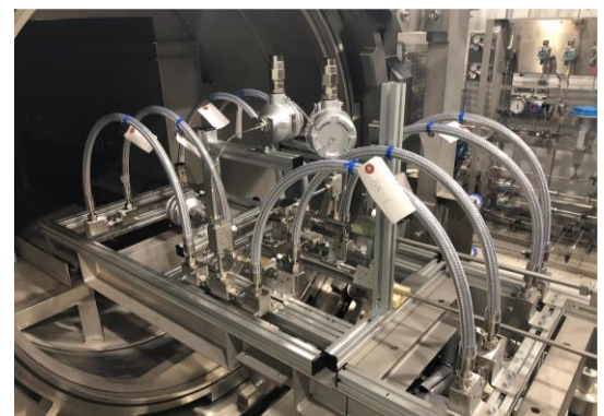
Hydrogen impulse test (durability test at Iwatani R&D Center)
