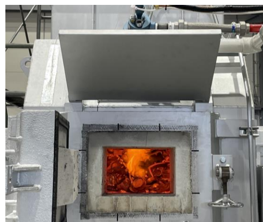
Aluminum melting test using hydrogen combustion
