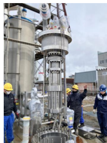
Liquid hydrogen pump featuring high efficiency and large flow rates, serving as a vital component of hydrogen infrastructure.
