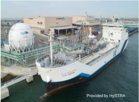
Liquid hydrogen carrier and cargo handling base
